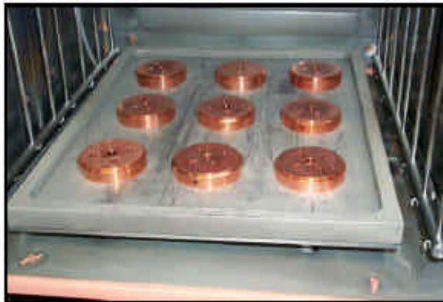
FXC Test Disks Stress Relieving
