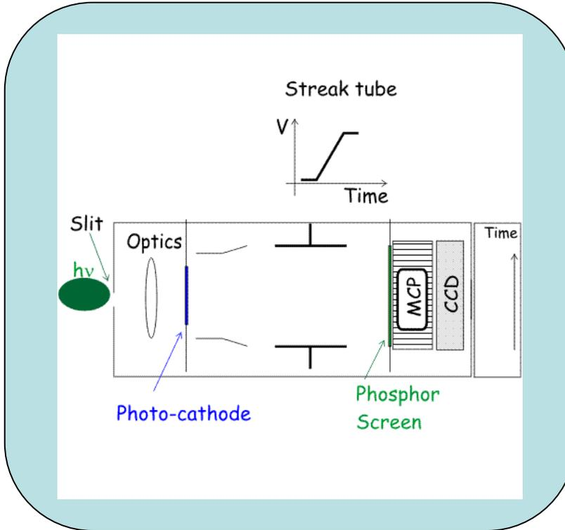
'Streak cameras uses a time dependent deflecting electric field to convert time information in spatial information on a CCD'
