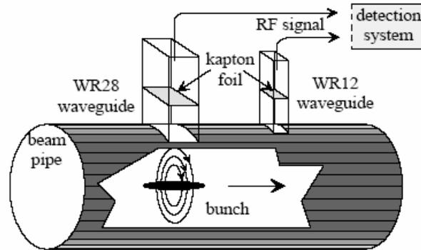
*'Based on the measurement of the bunch spectrum which is picked-up by a rectangular waveguide coupled to the beam pipe'*
