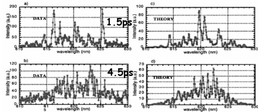
1.5ps. 200-500pC, 44MeV beam using a spectrometer with a resolution of 0.05nm/pixel
