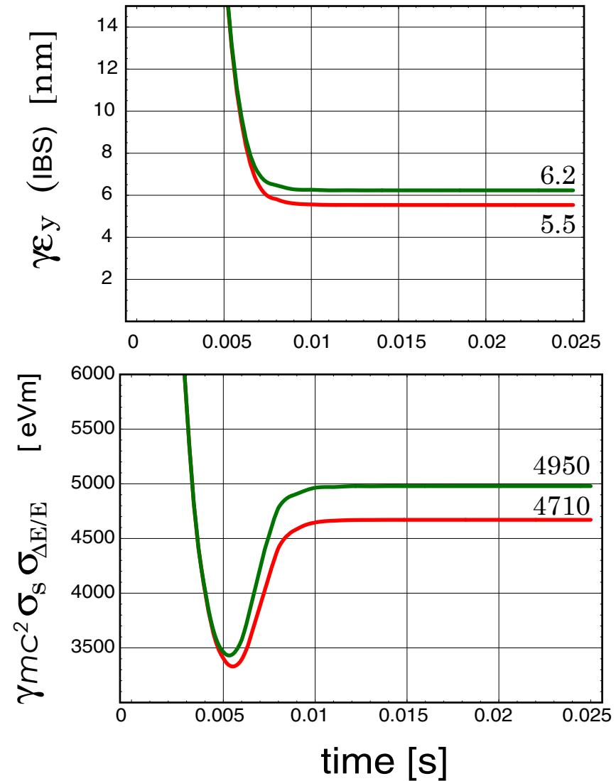
Emittance & bunch length evolution in CLIC\_DR with wiggler period of 10 cm at wiggler field of 0.5, 1.0, 1.5 and 2.0 T. Energy is 2.424 GeV, betatron coupling 1.1 %, bunch population  $4.2 \times 10^9$ , RF phase is constant.
