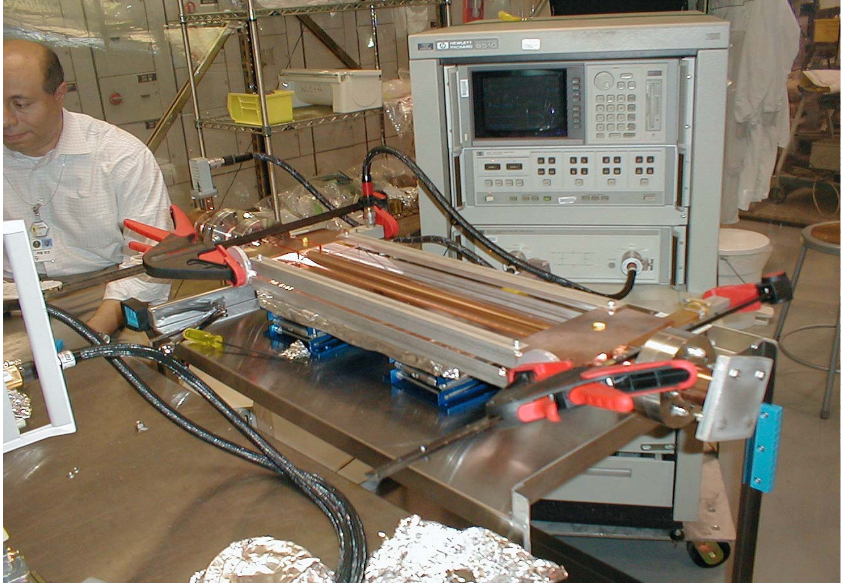
Directional Coupler Cold Test
