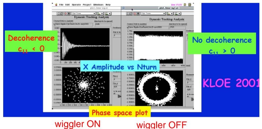
small negative c<sub>11</sub> is optimum for dynamic aperture & beam-beam
