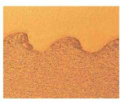
Photomicrograph of a typical explosion weld
