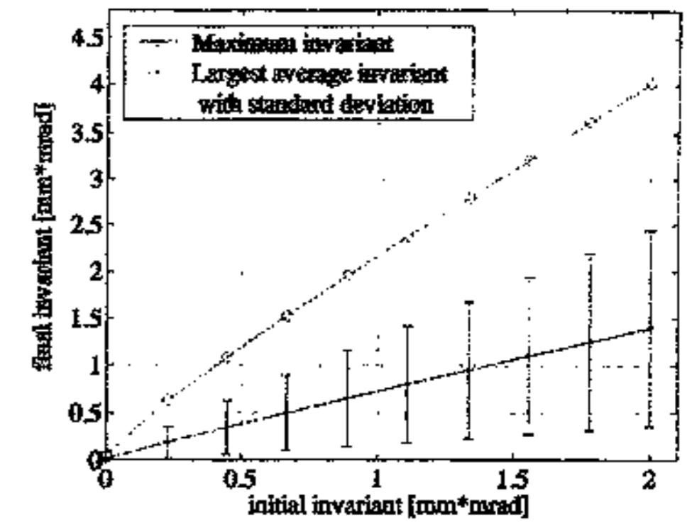
$I_{po\_max}$  and  $I_{po\_av}$  as a function of the injection Courant-Snyder Invariant
