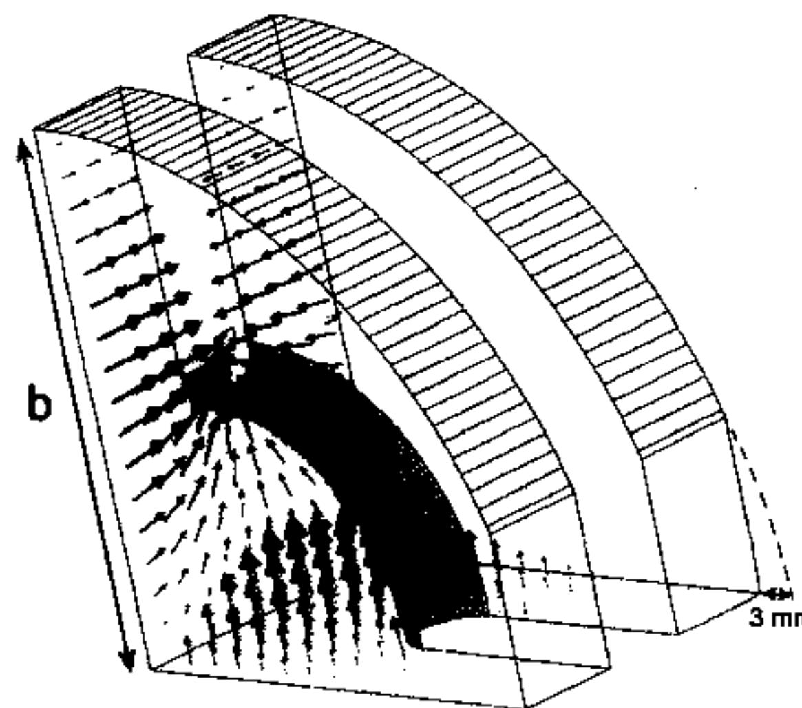
→ re-tuning of the fundamental mode by the sensitivities obtained by MAFIA (modified b radius)
