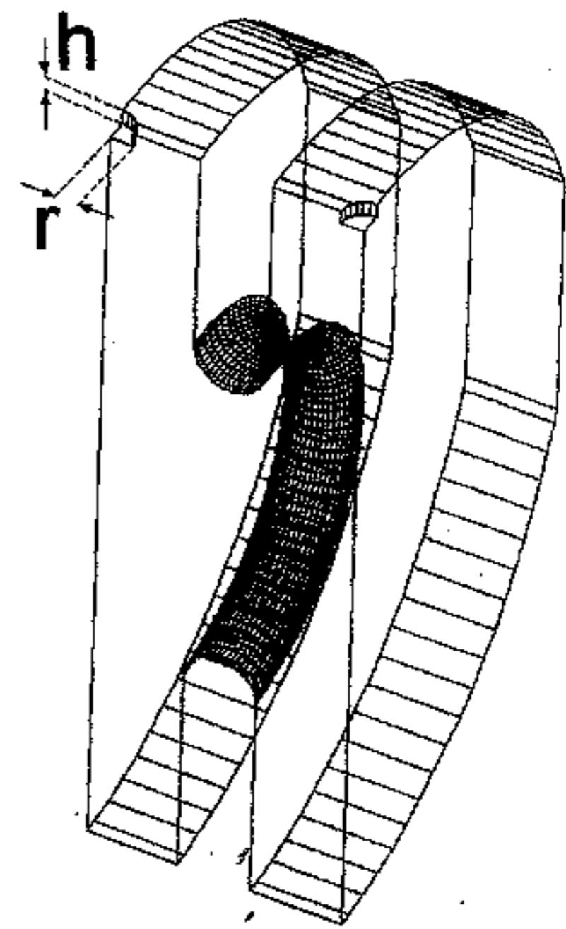
→ tuning of the single cell resonant frequency ( $r=3\text{mm}$ )
