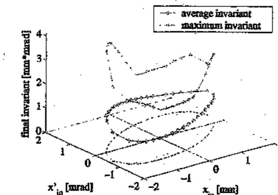
$I_{o-max}$  and  $I_{o-av}$  for a given  $I_{in}$  and various betatron phases
