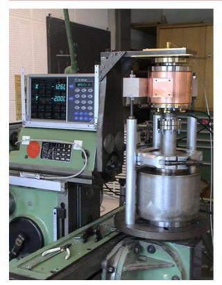
A thin wire forming a coaxial line was displaced diagonally across the pick-up aperture.
