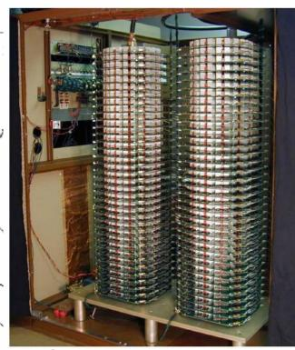
Assemblies of two parallel 35 serial switch stack assemblies for voltage and increased current capability
