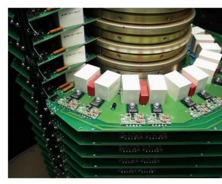
Partial view of parallel devices for current capability
