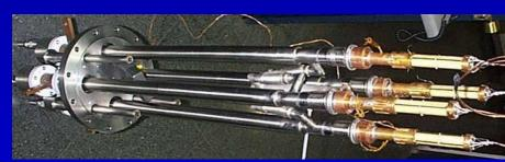
600 A hybrid current lead for LHC corrector magnets
