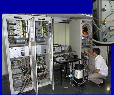
Modular control system based on µPs CAN network
