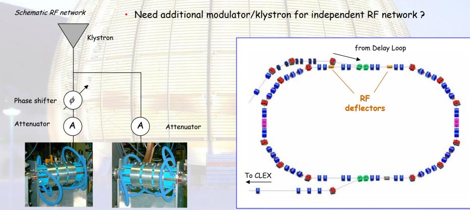
RF deflectors (INFN-LNF) installed during the Preliminary Phase
