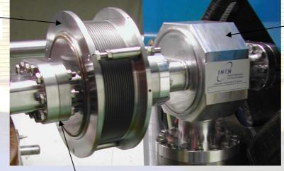
Special gasket profile for RF contact
