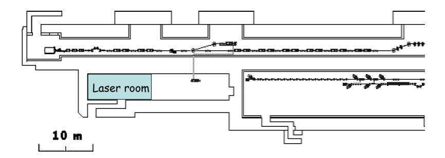
RF-Gun has to be at the beginning of the building due to the cathode loading system
