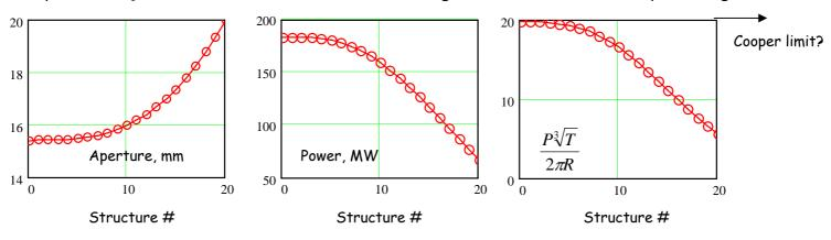
Example (a(n)= $a_0+\Delta a \times n^3/N^3$ ): 20 structures, 0.8 m long, total extraction 65 %, pulse length 140 ns
