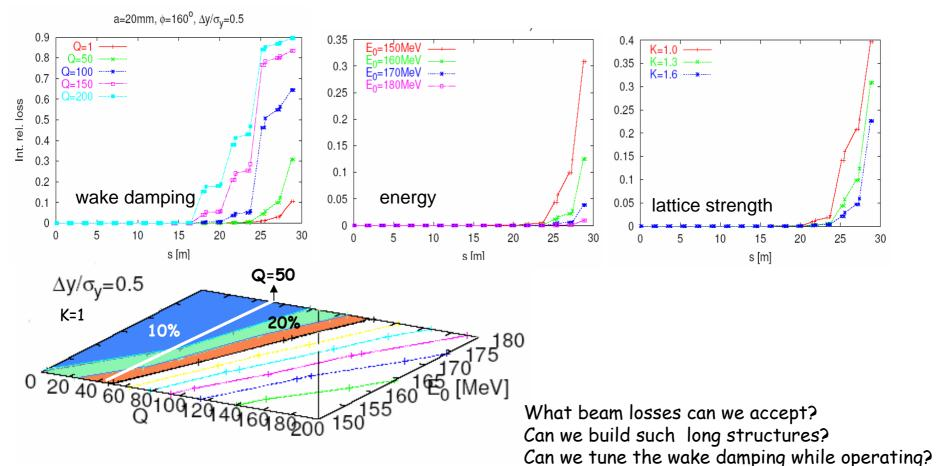
The beam energy and lattice strength do not give much room for tuning (all happened in the ~last structure) The change of beam current seriously affect extraction.
