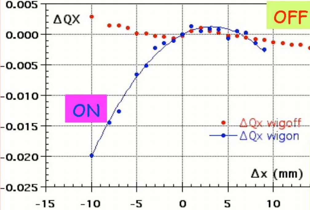
DAFNE horizontal tune vs. horizontal orbit offset with wiggler ON & OFF: *tune change 0.02 for orbit shift of 1 cm*
