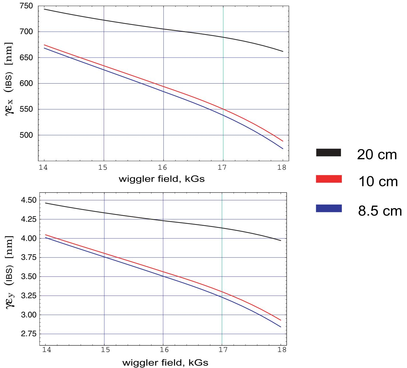
bunch length & energy spread dependence on wiggler field, bunch spacing 16 cm (1875 MHz)
