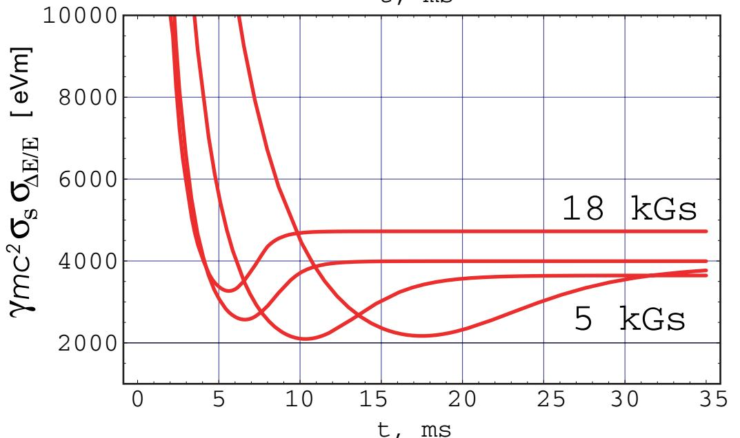
emittances dependence on wiggler field, bunch spacing 16 cm (1875 MHz)
