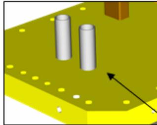
Water-cooling Connections (Ø16mm) Brazed to the cover plate
