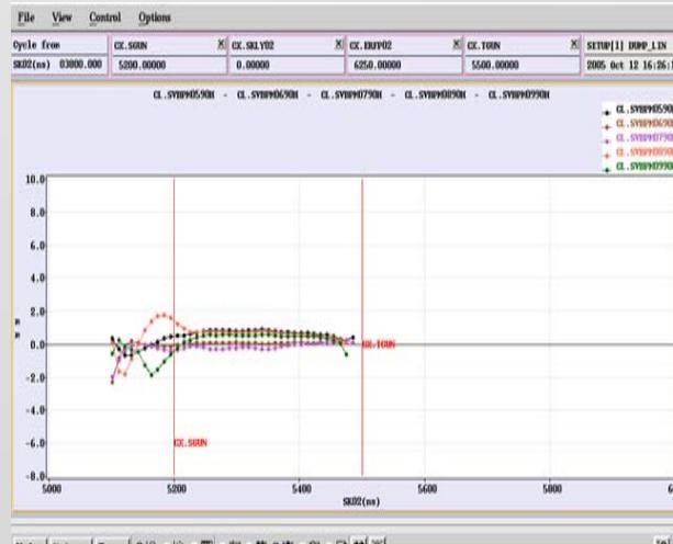
Horizontal beam position constant over the pulse.
