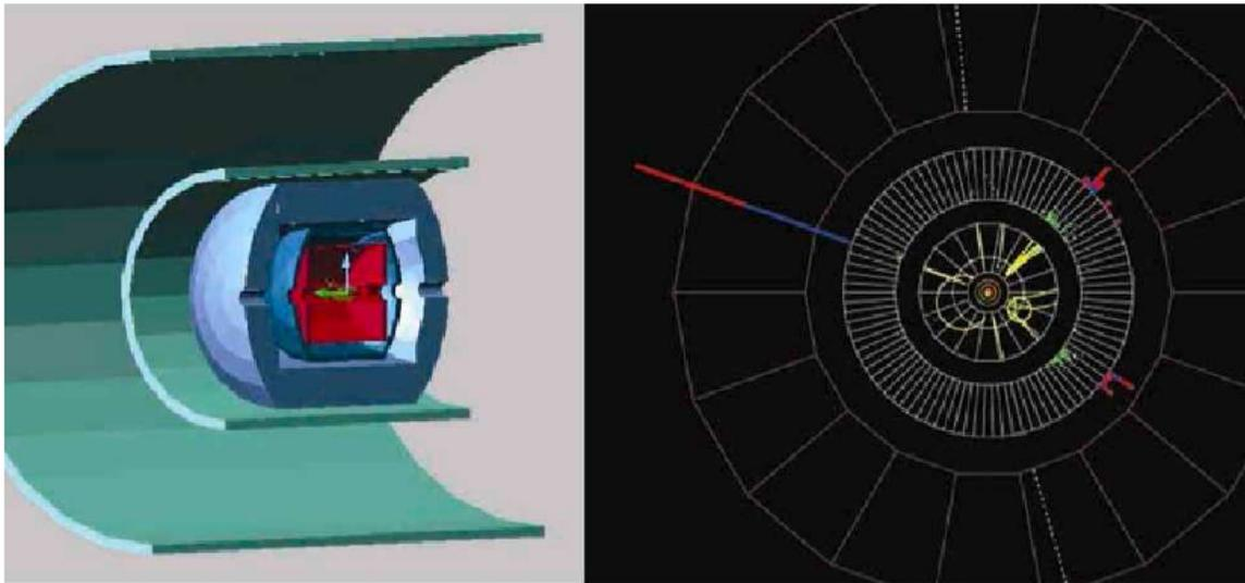
**Figure 1.** A drawing of the overall 4th Concept geometry showing the projective dual-readout calorimeter surrounding the tracking volume with the TPC, the inner solenoid at  $r = 3\text{m}$  outside the calorimeter, and the muon tracking volume in the annulus between the inner solenoid and the outer solenoid at  $r = 5.6\text{m}$ .
