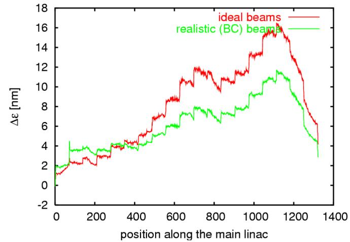
standard average misalignments, 2 test beams,  $\Delta\Phi = \pm 10 / E = 0.8, 0.9 E_0$ ,  $G = 0.8$ ,  $\omega = 100$ , average of 50 machines, best final emittance growth 2.8 nm
