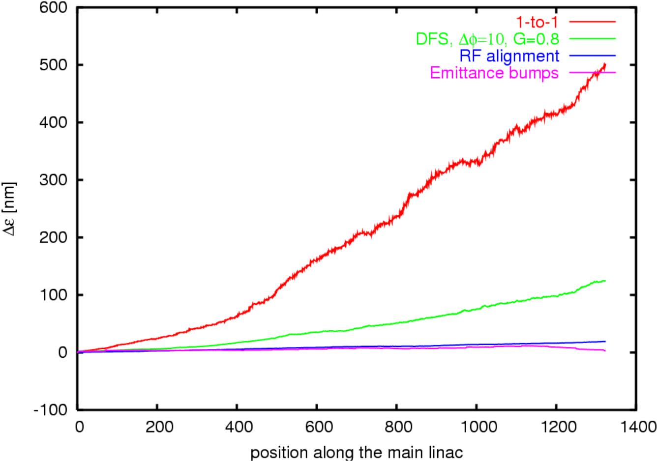
standard average misalignments, 2 test beams,  $\Delta\Phi = \pm 10$ ,  $\omega = 100$ ,  $G = 0.8$ , average of 50 machines, final emittance growth 2.8 nm
