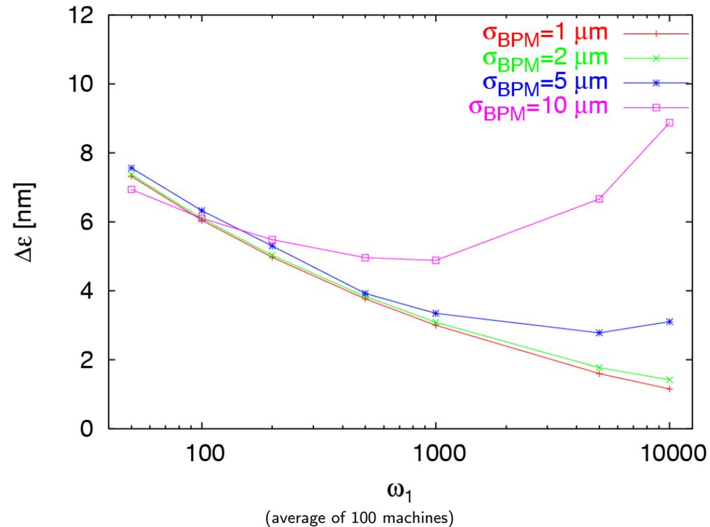
for a laser-straight linac, DFS (with  $\omega$  "big", BPM resolution of 1  $\mu\text{m}$ ) leads to excellent results
