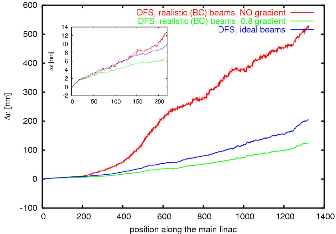
standard average misalignments, 2 test beams,  $\Delta\Phi = \pm 10$ ,  $G = 1.0, 0.8$ ,  $\omega = 100$ , average of 50 machines
