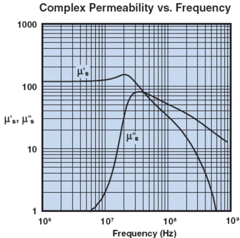
Measured on a 19/10/6mm toroid using the HP 4284A and the HP 4291A.
