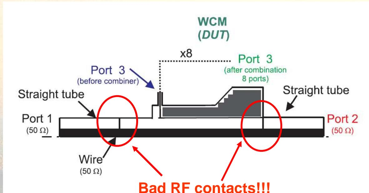
The experimental setup showed very bad RF contacts between WCM and the two external straight tubes. In order to improve the contacts some pasty stripes of conducting material has been used.... Unfortunately it cannot be used in vacuum....
