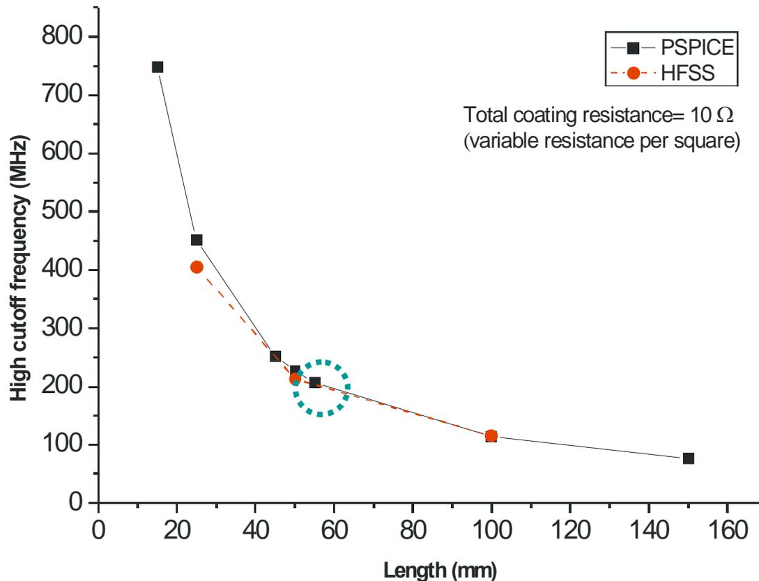
The smaller the length the higher the high frequency cutoff.
