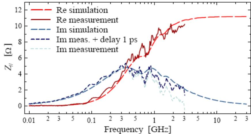
M. GASIOR, LIMITING HIGH FREQUENCY LONGITUDINAL IMPEDANCE OF AN INDUCTIVE PICK-UP BY A THIN METALLIC LAYER, CERN-AB-2004-090
