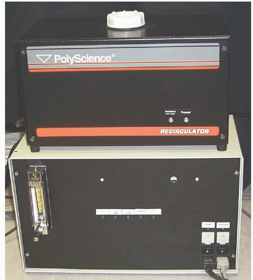
Water cooling system and integration electronics
