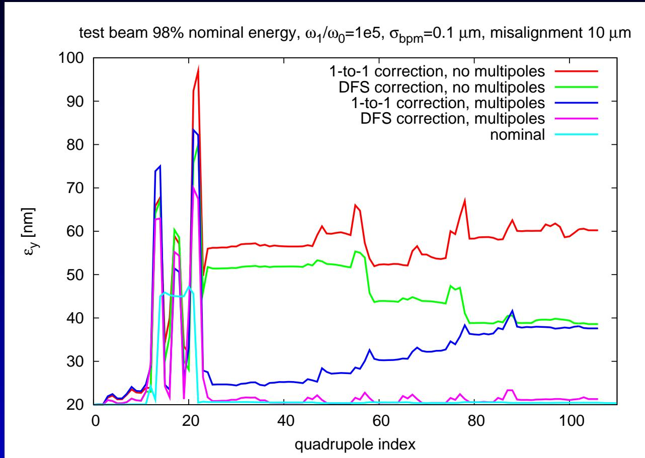
5% emittance growth after aligning only the collimation section.
