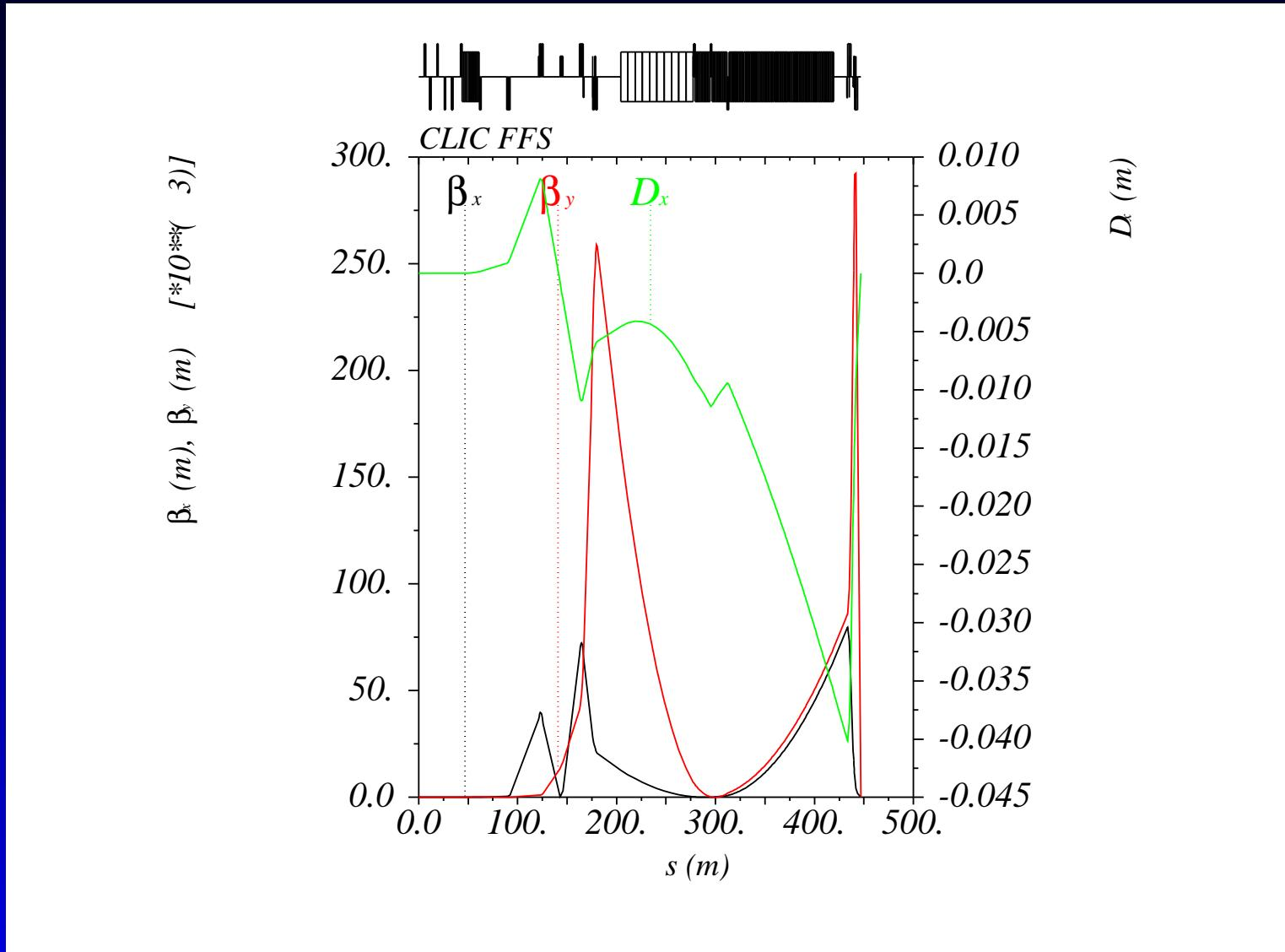
$$\beta_{IP,x} = 7\text{mm}, \beta_{IP,y} = 0.067\text{mm}$$
