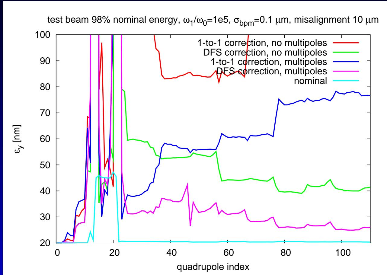
Does not work. The FFS corrupts the correction in the collimation section.
