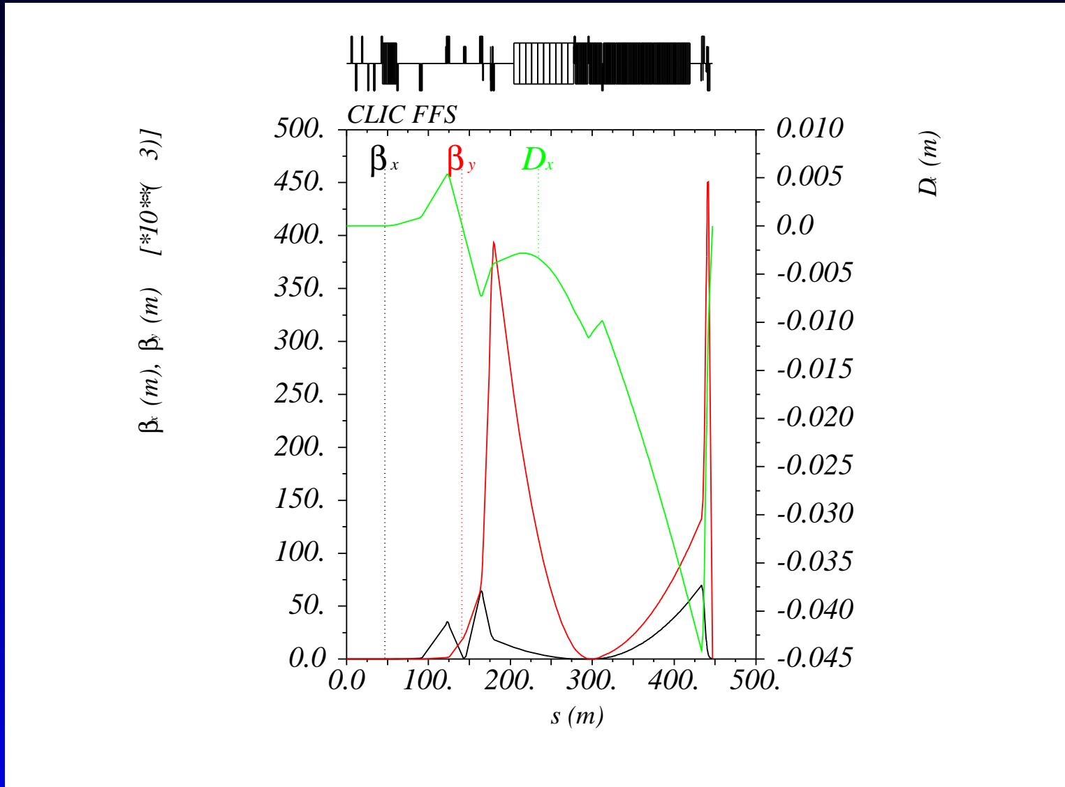
$$\beta_{IP,x} = 8\text{mm}, \beta_{IP,y} = 0.045\text{mm}$$
