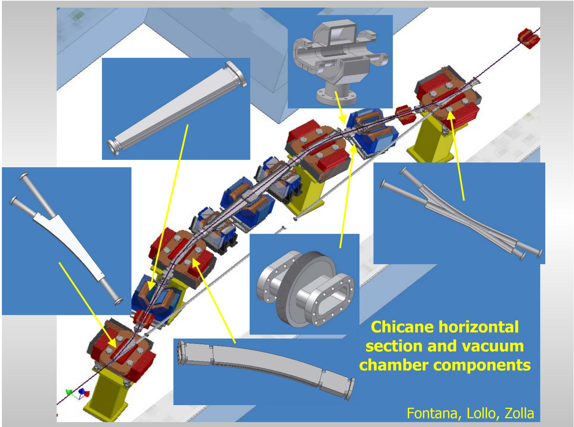
**Chicane horizontal section and vacuum chamber components**
