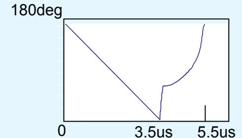
The arbitrary waveform generator houses the phase program for the pulse compression and the frequency offset. The function looks like shown in fig. above for a positive frequency offset. For a negative frequency offset the function is a mirror image of that one. The clock frequency can be the same as the one used for the data acquisition system.
