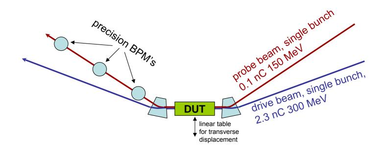
With BPM's spaced by 4 m, 10  $\mu$ m BPM resolution and 1 mm space to move the DUT transverse wakepotentials of  $\geq$  10 $\mu$ m/4m·150MeV/2.3nC/1mm =
