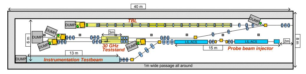
Beam line layout in CLEX is intimately linked with layout and functionality of TL2
