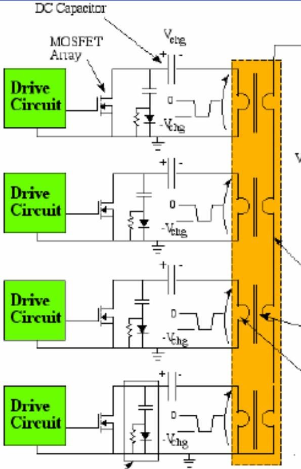
Pulse generator schematic
