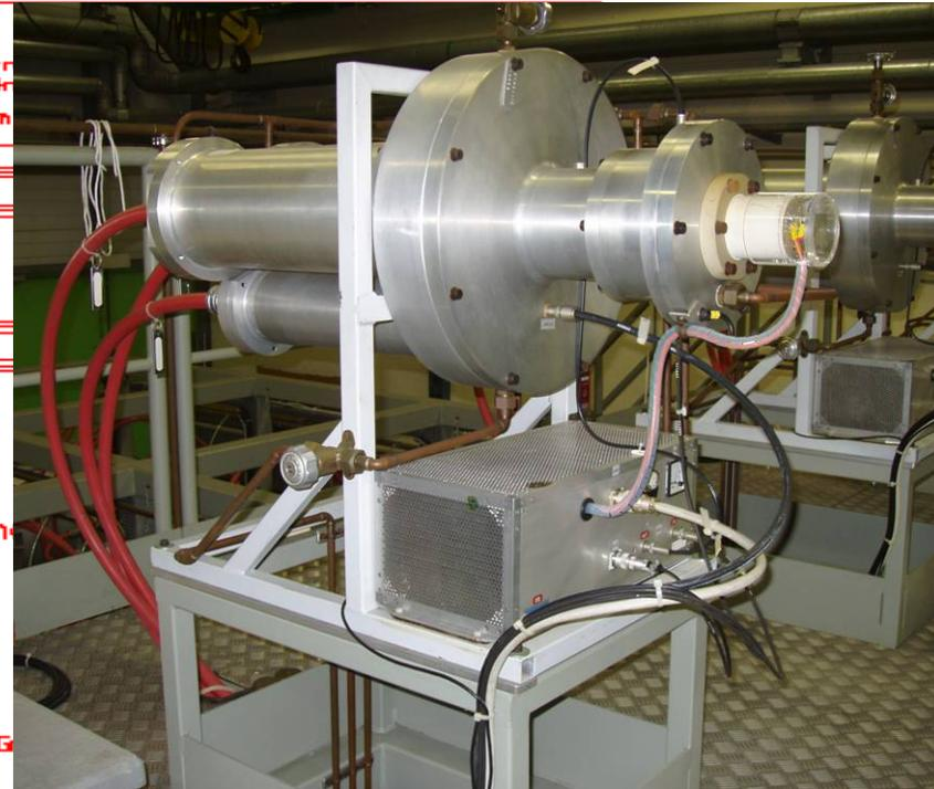
Dump switch with terminating resistors
