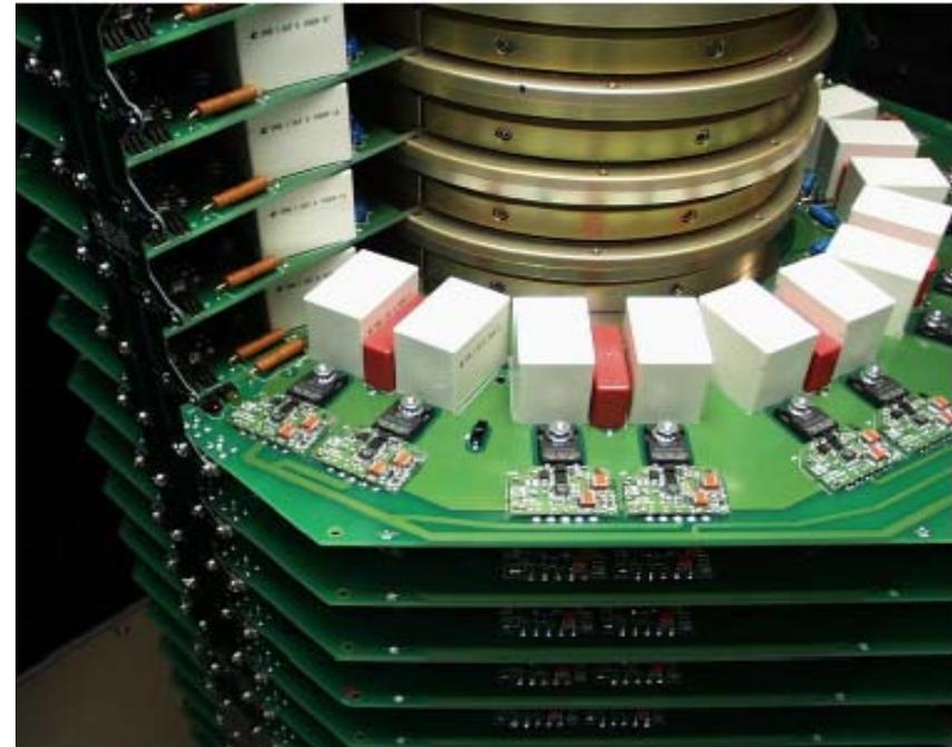
Partial view of parallel devices for current capability
