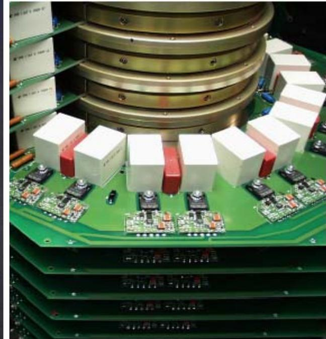
Partial view of parallel devices for current capability
