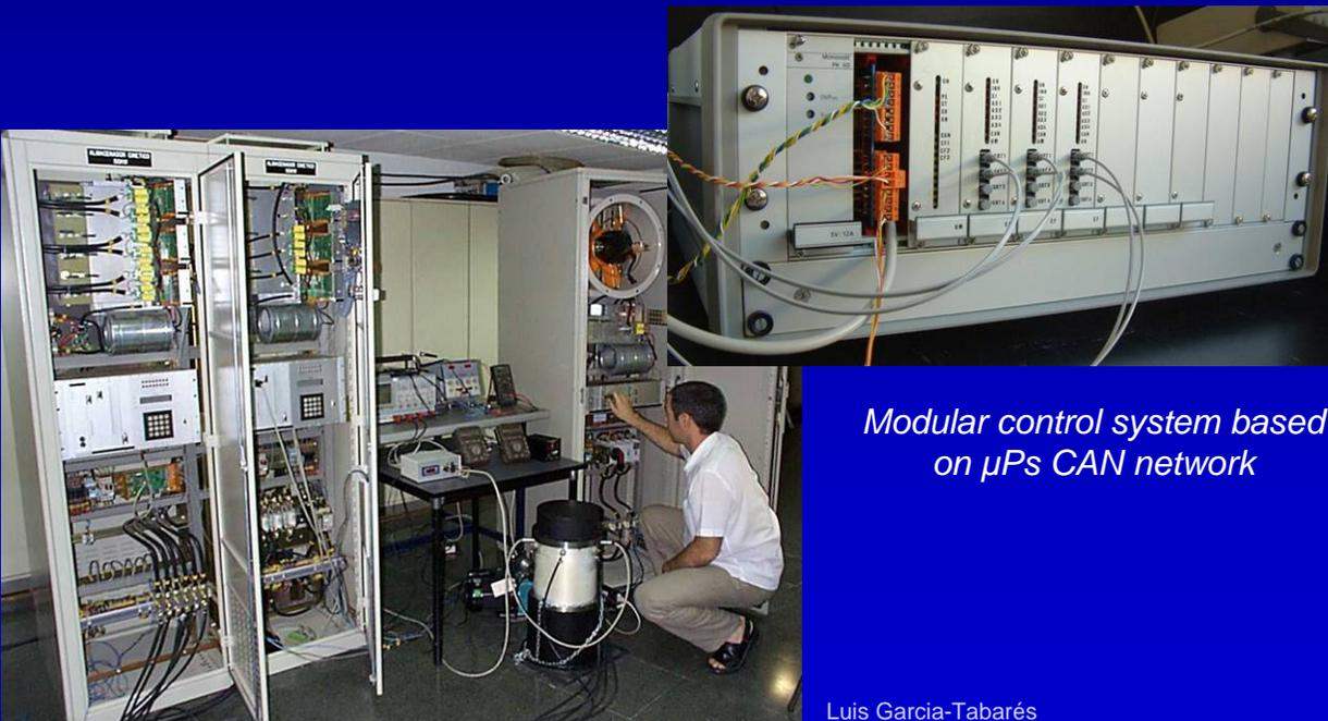
*Modular control system based on  $\mu$ Ps CAN network*
