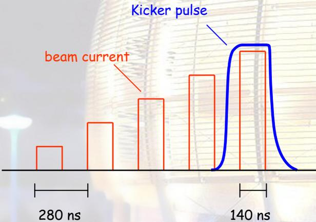
Evolution of beam current circulating in the ring over 5 turns & kicker pulse
