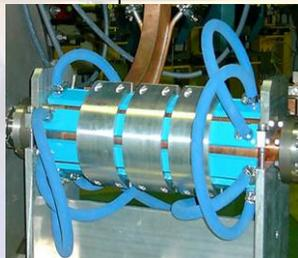
RF deflectors (INFN-LNF) installed during the Preliminary Phase
