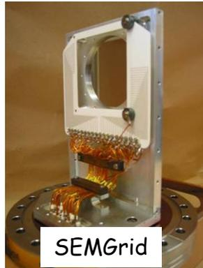
New support to avoid mechanical stress induced by the beam
