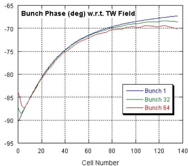
$\Delta\phi_b = \Delta\omega T = 6^\circ$  between 1st and last bunch
