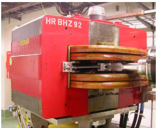
Type BHF: ex-EPA dipole with field gradient
