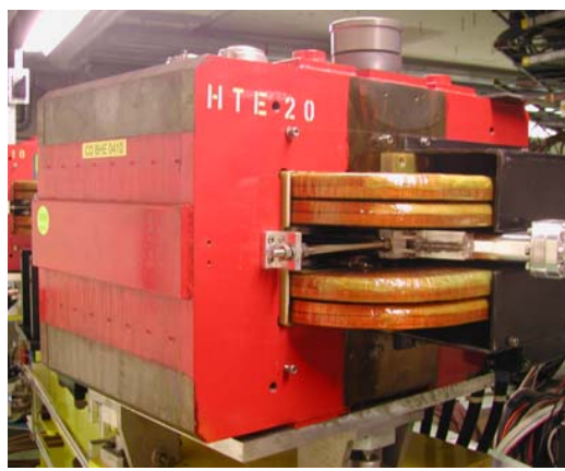
Type BHE: ex-EPA dipole with pure dipole field
