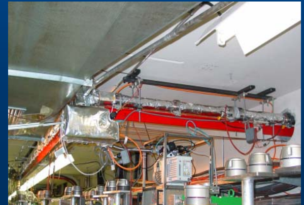
30 GHz transfer line. Transfer Efficiency 85%.
