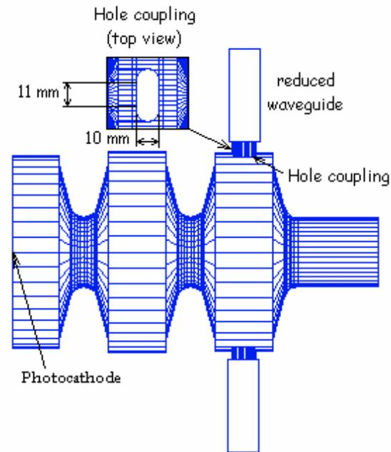
$$Q = 14400, R_s = 7.84 \text{ M}\Omega \Rightarrow P_{\text{HF}} = 5.2 \text{ MW} \text{ for } 80 \text{ MV/m}$$
