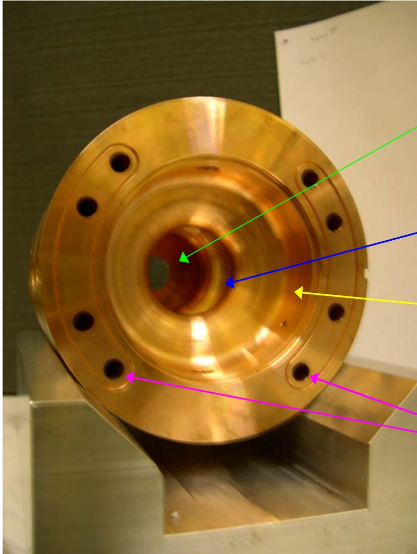
First half cavity with the hole for the photo-cathode
