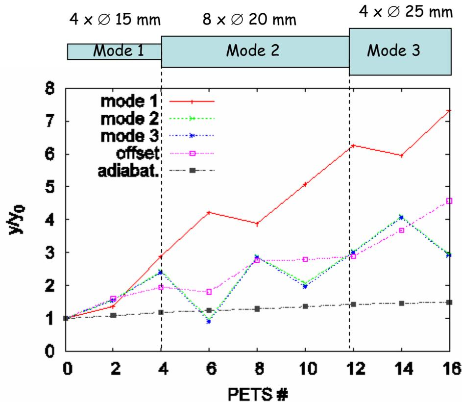
For this configuration we can expect stable operation (no beam losses) and relatively high beam power extraction.
