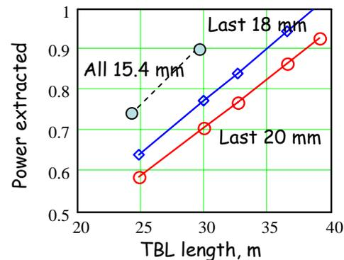
Note, if the structure length were to be a free parameter, than for the constant aperture TBL, the total length ~30 m will be optimal to extract 90% power.
