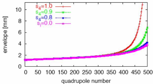
The mode #4 can cause the beam losses in the CLIC drive beam decelerator
