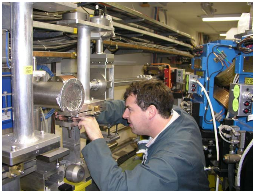
Alignment of a CERN BPM
